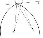
Consider the support line  $\ell$  orthogonal to bisector of  $\widehat{aqb}$  at the point q. It can be slightly rotated remaining support at the point q. We find point  $\tilde{q} \in \ell$  such that  $|\tilde{q} - a| = |\tilde{q} - b|$ .
